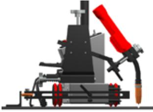
The MOGGY® is ideal for butt joint welding. Here the MOGGY® is using a fence to guide it accurately along the desired path. Standard v- groove track can also be used.
