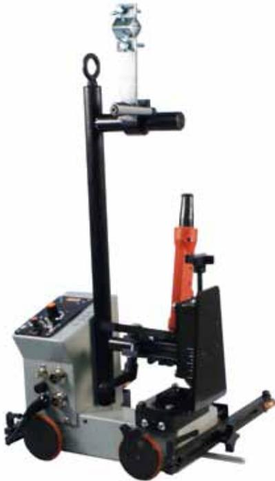
Ideal for automatic horizontal fillet, lap or butt welding applications
