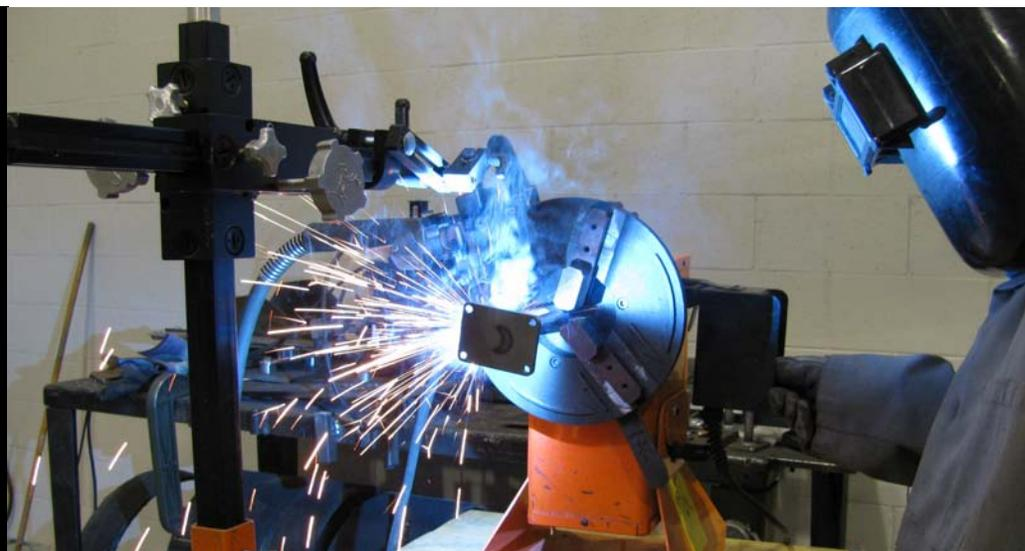
GP/GPP 200 SERIES POSITIONERS ARE AVAILABLE IN STANDARD OR PROGRAMMABLE MODELS WHICH ARE EQUIPPED WITH CORRESPONDING REMOTE CONTROLS
