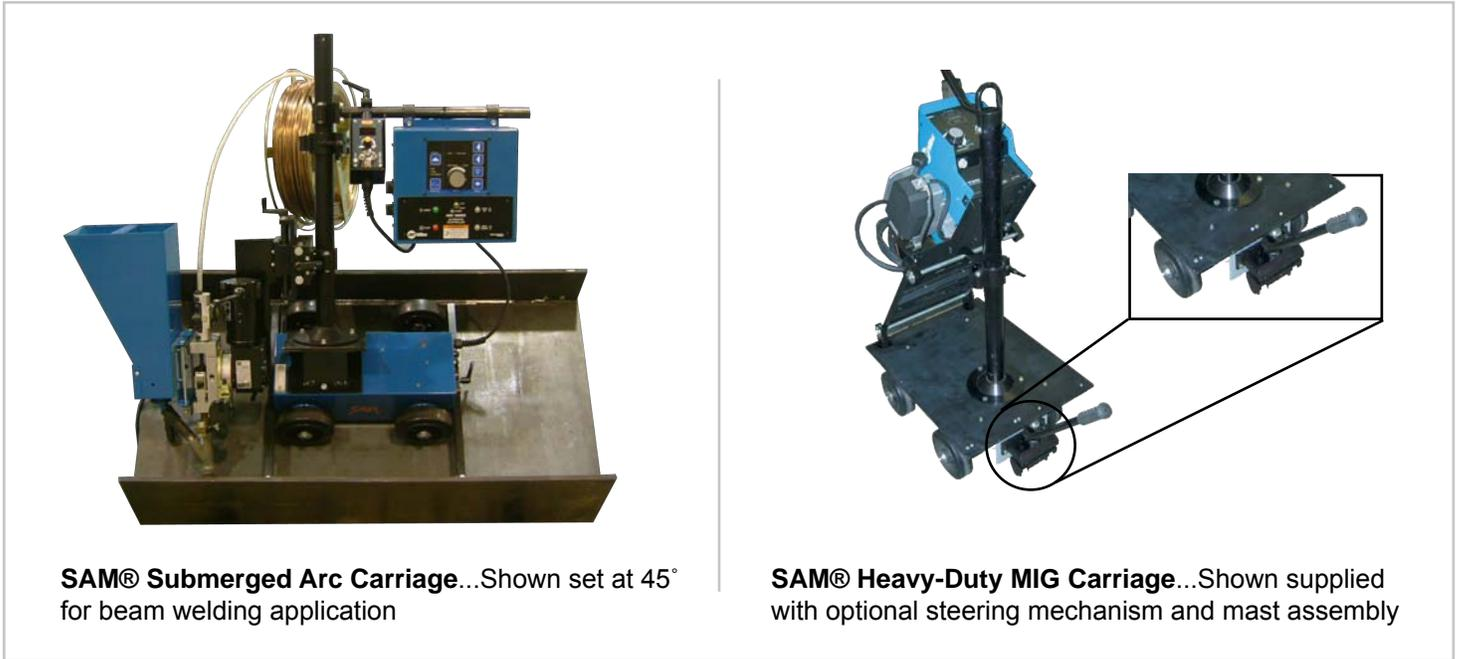
**SAM® Submerged Arc Carriage**...Shown set at 45° for beam welding application
