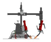
Dual gun holder assembly mounted on the Moggy enables positioning of 2 guns and simultaneous activation of two wire feed signals. Moggy is guided by the workpiece.
