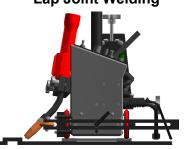
The Moggy is performing a lap joint weld. It is guided by Industry Standard 6" (152.4mm) v-groove Track running parallel to the joint.
