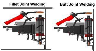
EFFICIENT...EFFECTIVE...VERSATILE The Gullco magnetic moggy is highly versatile and is ideally suited to a wide variety of welding applications, particularly in Tee fillet welding where there is not enough room for the carriage to run on the horizontal plate.
